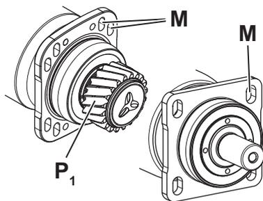
The gearbox can be optionally equipped with an output pinion [P<sub>1</sub>]. The gearing backlash between output pinion and toothed rack/counter-wheel can be adjusted using the slotted holes [M] and the lateral guides. An additional adjustment mechanism is no longer necessary.
