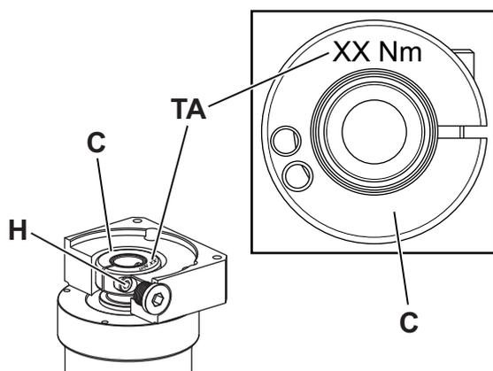
The tightening torque value [TA] of the clamping bolt [H] can be found on the clamping hub [C].
