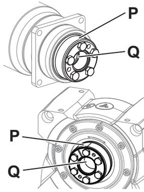
The slip-on shaft / hollow shaft / hollow shaft interface [Q] is axially secured to the load shaft by means of a shrink disk connection. If a gearbox with shrink disk [P] was ordered, then it is already mounted.
